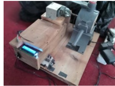
Fig. 5. Photograph of the Design Results for the Miniature Disk Mill Monitoring Machine
